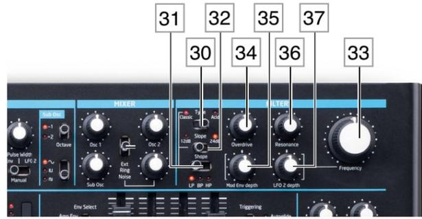
The sum created in the mixer from the various signal sources is fed to the Filter Section. Bass Station II's filter section is both simple and traditional, and can be configured with only a small number of single-function controls.
